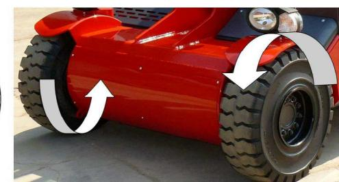
front wheel drive with 2 motors and counter rotation - total steering
